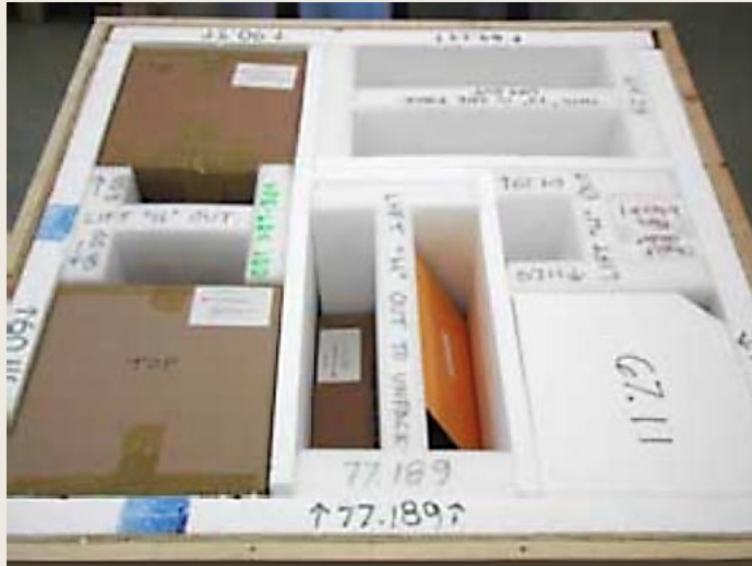
Interior of hard shell crate with PE foam partitions to secure inner boxes
