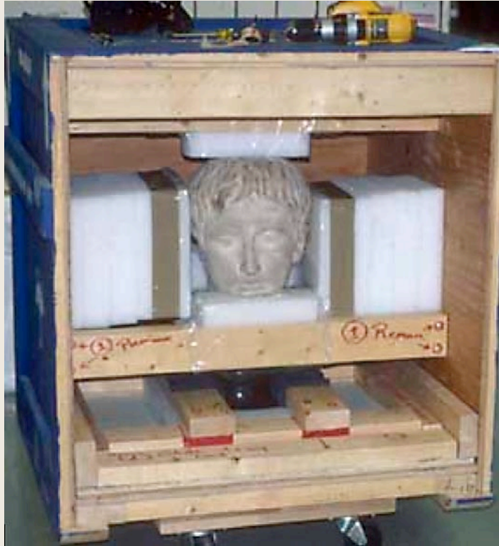
Hard shell crate with removable bottom tray and PE foam blocks attached to inner walls. Screws for uncrating are clearly marked in order of importance
