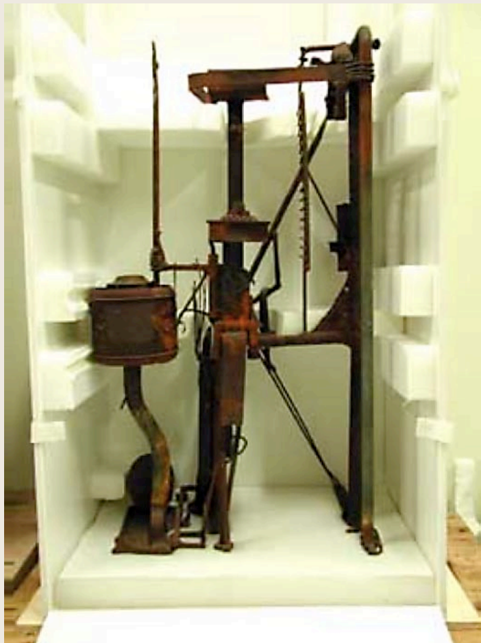
Collared cut-outs of PE foam lined with cross-linked PE foam sheet in half-inch foam core box
